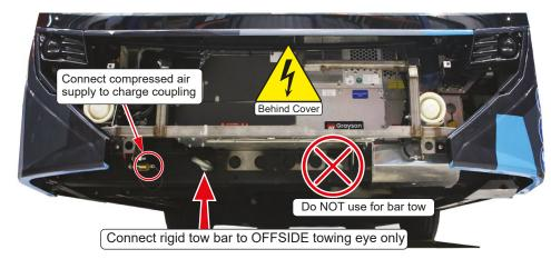
For rigid bar towing, only the OFFSIDE eye must be used, as indicated, to prevent damage to the front components.
