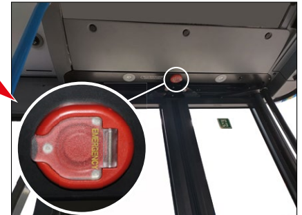
Internal Emergency Exit Button
