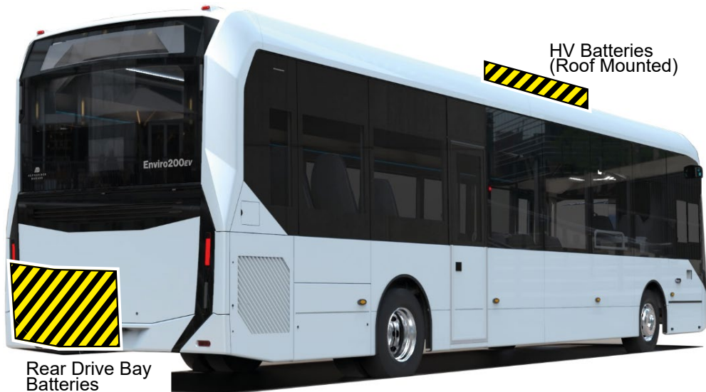
Left hand rear side battery locations
