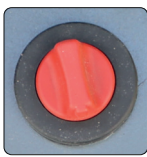
Rear External Emergency Stop Switch
